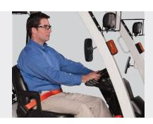
**High Visibility Seatbelt**Bright orange seatbelt provides instant visual confirmation that operators are using this safety equipment.
