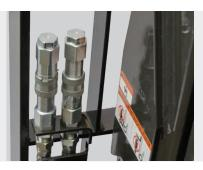
Hydraulic Quick Disconnect Simplifies change-out when multiple attachments are used to get your forklift back in operation quicker.
