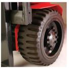
Flexi AC 1200 front twin drive wheels provide excellent grip and traction in slippery conditions when fully loaded. Continental MC20 super-elastic finger tread tyres for extended service life and resistant to damage.
