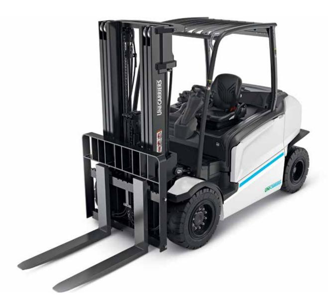
**Electric Pneumatic Tire Lift Truck**
