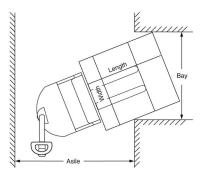
Aisle dimensions listed above assume 4" between loads. Use the larger dimension; load width or load length. For ease of use and add 6" to 12" for operator clearance to the appropriate specifications listed above. Truck performance may vary due to application requirements' and changes in model design.
